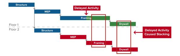
Furthermore, trade stacking on top of delays does not reflect a feasible reality, especially considering the overbearing amount of resource and crew restraints happening in the built environment right now. Additionally, when activities automatically stack on top of each other, float becomes consumed. And, when float is consumed, everything becomes compressed by design.
