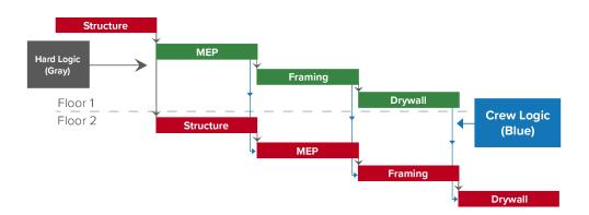
Now, the schedule has crew logic (featured in blue) embedded within it. The crew logic notifies the scheduling program that, for example, you cannot start framing on floor two until the framing is complete on floor one.
