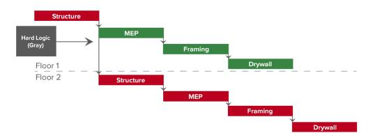
The hard logic in this CPM schedule is explaining that you cannot begin Mechanical, Engineering, and Plumbing (MEP) work on floor one until you have completed the structure on level one. Similarly, you cannot start the structure of the second floor until you are done with the first floor's structure because you cannot build on thin air; you need the structure below to do so.
