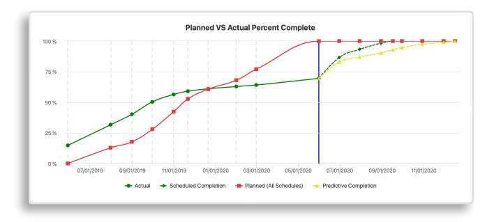
As depicted in the graph above, the project's progress curve is extrapolated by using the SPI to adjust the scheduled completion, shown by the yellow line. The yellow line is the schedule forecast, predicting the project will be 100% completed about four months later than what the scheduled completion date is telling you and six months later than the baseline plan indicated.
